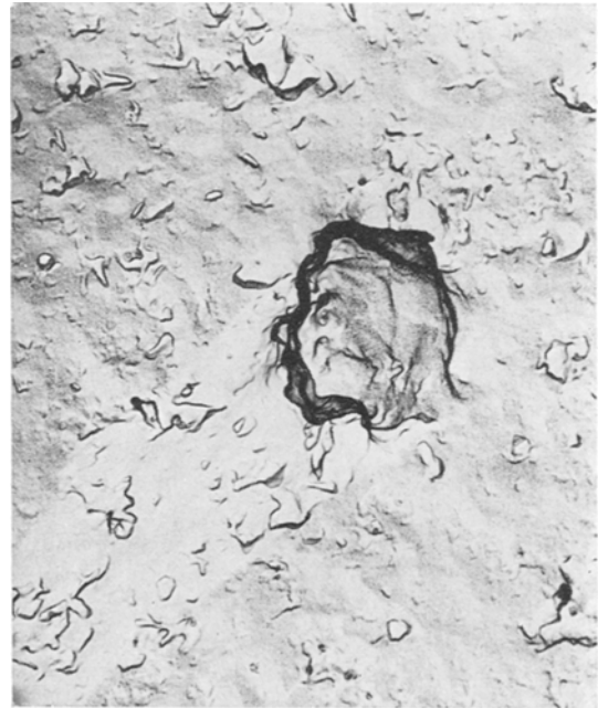
Figure 4 Microporosities in as-extruded SAP ( \times 20000 ).
